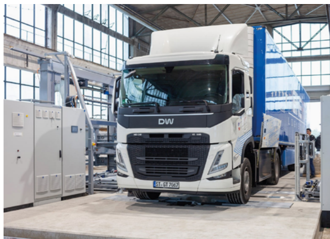
Figure 5: Battery swapping station from the e-Haul project and a prototype of the swapping module for trailers by Trailer Dynamics (Image: TU Berlin, Sustainable Truck&Van)
