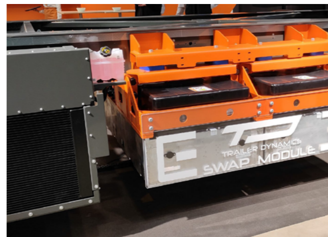
Figure 5: Battery swapping station from the e-Haul project and a prototype of the swapping module for trailers by Trailer Dynamics (Image: TU Berlin, Sustainable Truck&Van)
