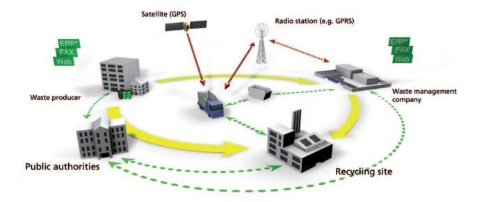
Telematics means the combination of technologies from the sectors of »telecommunication« and »computing science«. Due to the combination of information in different EDP systems via telecommunication and data processing solutions telematic systems create a new type of approach to the improvement and optimization of processes, planning and control in logistics and transportation.
