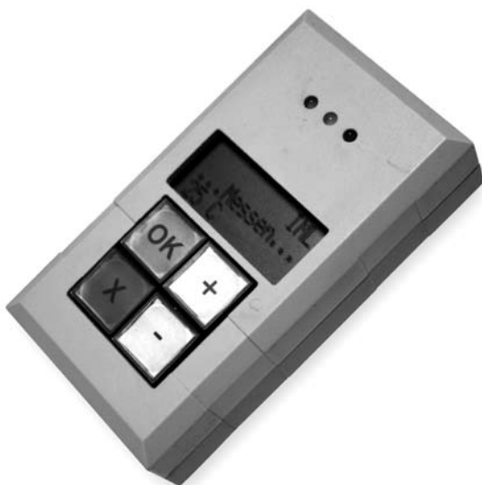
Prototyp des drahtlosen Pick-to-Light-Systems. Prototype of the wireless pick-to-light system.
