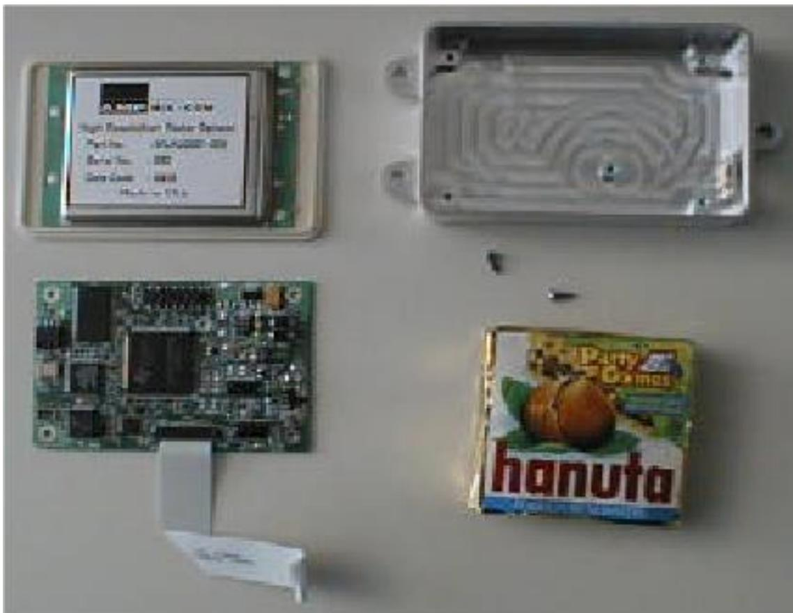
**Abb. 6: Tyco SLR C3 Radar-Sensor**
